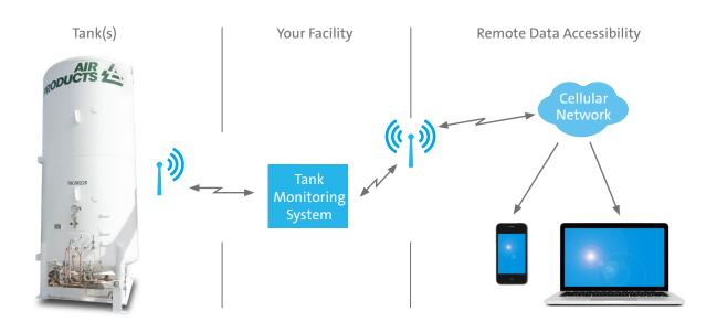
Installation includes differential pressure measurement and an optional pressure transmitter at the tank, along with a Wireless Intelligent Node (WIN). The WIN takes tank readings at preset intervals (typically 1-2 min) and transmits the data wirelessly to an indoor receiver (gateway). Each WIN can handle two tanks and there is no limit to the number of tanks that can be monitored at a facility.
