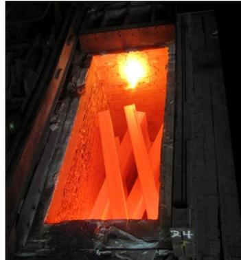
Figure 2: Photograph of a soaking pit furnace at ArcelorMittal's facility in Steelton, Pennsylvania
