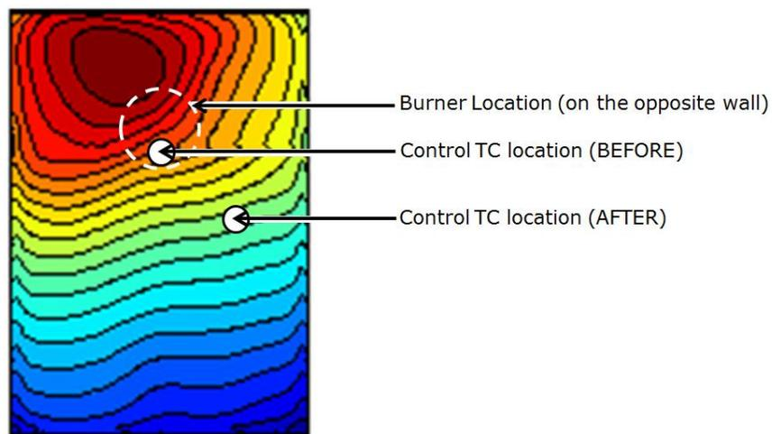
Figure 4: CLOP output ranking the locations for placement of control thermocouple for most effective control strategy. Red = worst location to Blue = best location.
