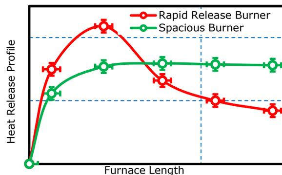
Figure 1: Heat release profiles for different types of Air Products oxy-fuel burners measured under controlled conditions in a test furnace
